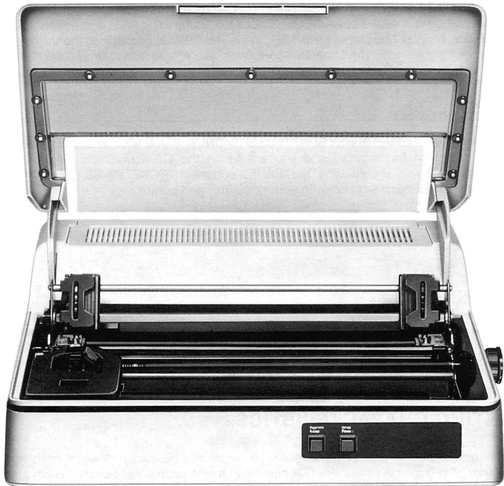
Figure1. Feed Mechanism and Ribbon Cartridge
